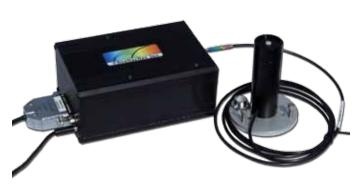
Spectrocolorimeter: Measures the color of reflected light. Simultaneous window (with live spectra) displays 1976 CIE LAB diagram for L\*, a\*, b\*. Display CIELAB color values with chroma, hue, x, y, and tristimulus and Delta-E\*. Load or save standards for subsequent Delta-E\* color comparisons.
